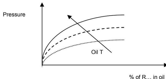
The diagram above illustrates a specific property [Charles' Law] of gases, which are more soluble in liquids as the pressure increases but less soluble as the temperature increases: if the oil in the sump is held at a constant pressure, an increase in oil temperature will significantly reduce the amount of refrigerant dissolved in it, thus ensuring that the lubricating function desired is maintained.
